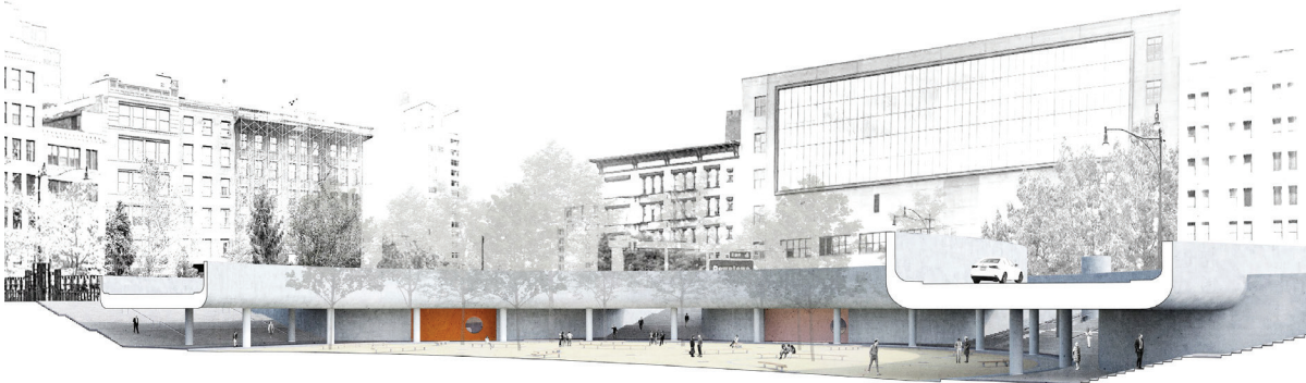
Perspective section showing pedestrian flow from street to central sunken park with roadways above and interior program spaces beyond.
